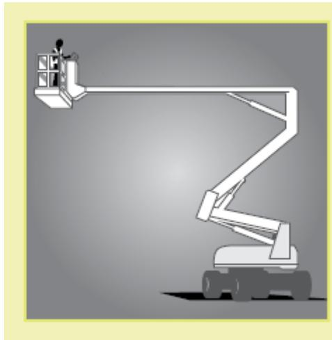
An example of a boom-type elevating work platform. The safety harness and lanyard assembly are not shown for purposes of clarity. The lanyard should be as short as possible and should be attached directly to the designated anchor point on the EWP, not to the handrail.
